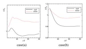
Figure 11: Streamwise entropy distribution
