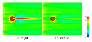
Figure 7: Contours of Nu number on x - z plane
