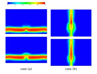
Figure 10: Mean scalar field on the x - y plane (upper: rigid; lower: elastic )
