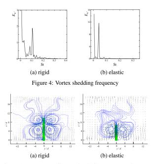
Figure 5: Mean streamlines and velocity vectors on the x - y plane
